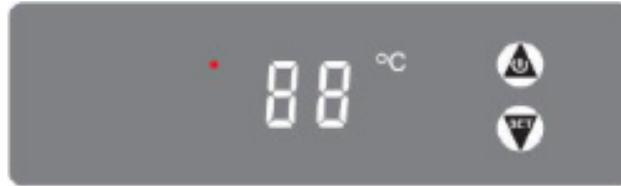
1. Press the “up arrow” and hold for 3 seconds to turn the electric heater ON/OFF. When the heater is turned OFF, it shows “- -”.
